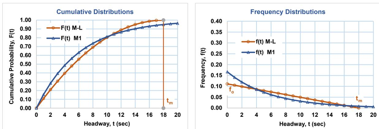
**Figure 6 - Cumulative distributions and frequency distributions for linear (M-L) headway distribution function (negative exponential (M1) distribution included for comparison)**
