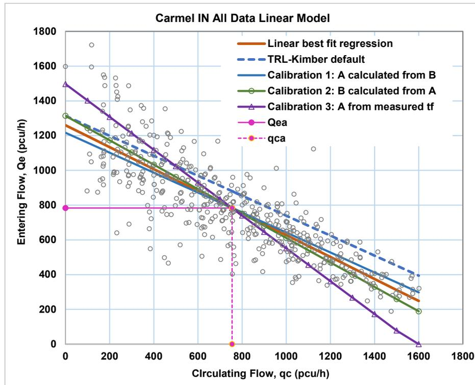
Figure 13 - Various methods of calibration of linear gap acceptance capacity models applied to the TRL linear model
