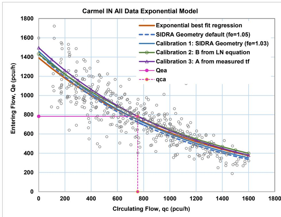
Figure 14 - Various methods of calibration of linear gap acceptance capacity models applied to the HCM (Siegloch M1) exponential model with basic SIDRA geometry method
