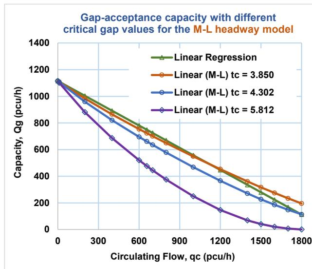
**Figure 9 - Comparison of the gap-acceptance capacity model based on the linear headway distribution (M-L) with a basic Linear model from regression using the HCM roundabout capacity research data using different critical gap,  $t_c$  values**
