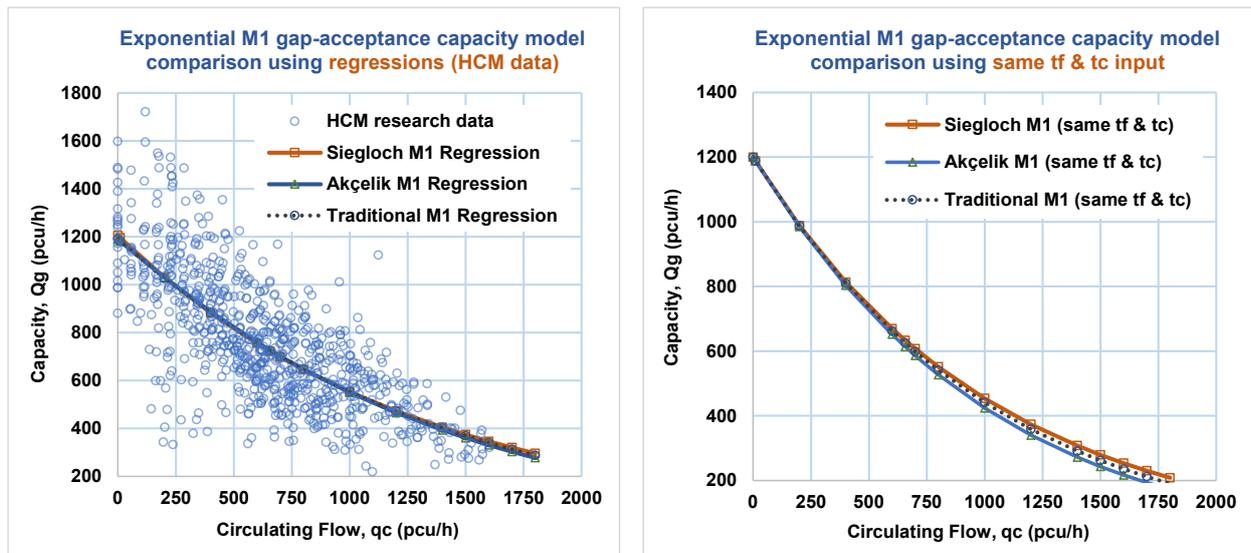
**Figure 3 - Comparison of three exponential capacity models based on the simple negative exponential (M1) headway distribution**
