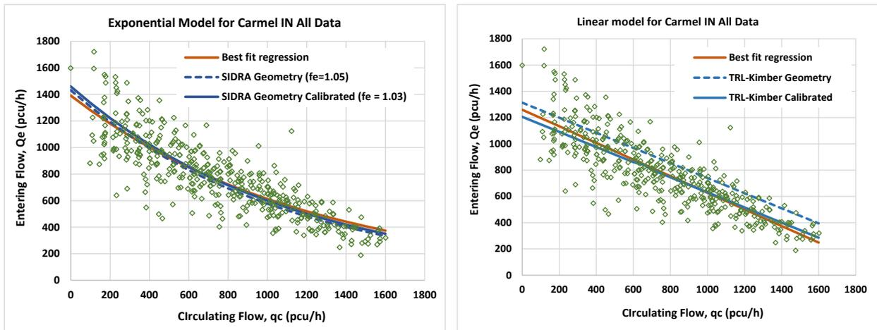
Figure 11 - Capacity data and estimates from regressions, HCM (Siegloch M1) Exponential model with SIDRA Basic Geometry method and TRL-Kimber Linear model
