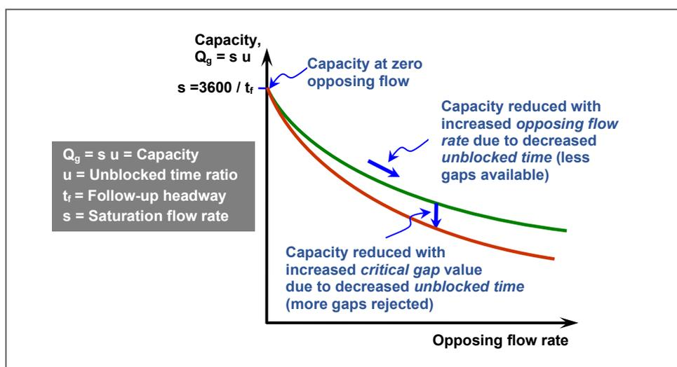
Figure 7 - Gap acceptance capacity
