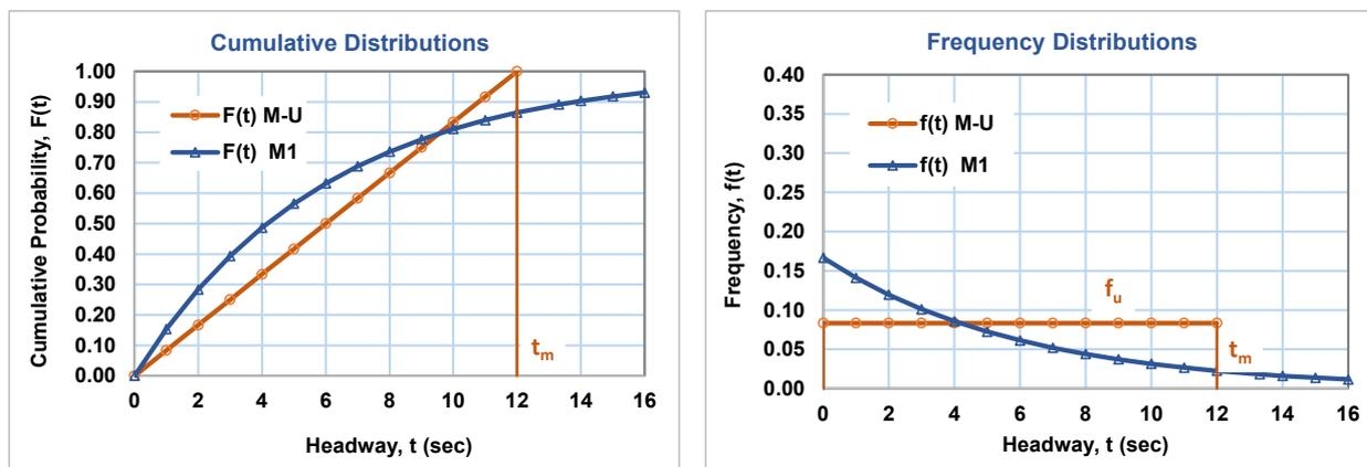
**Figure 5 - Cumulative distributions and frequency distributions for uniform (M-U) headway distribution function (negative exponential (M1) distribution included for comparison)**
