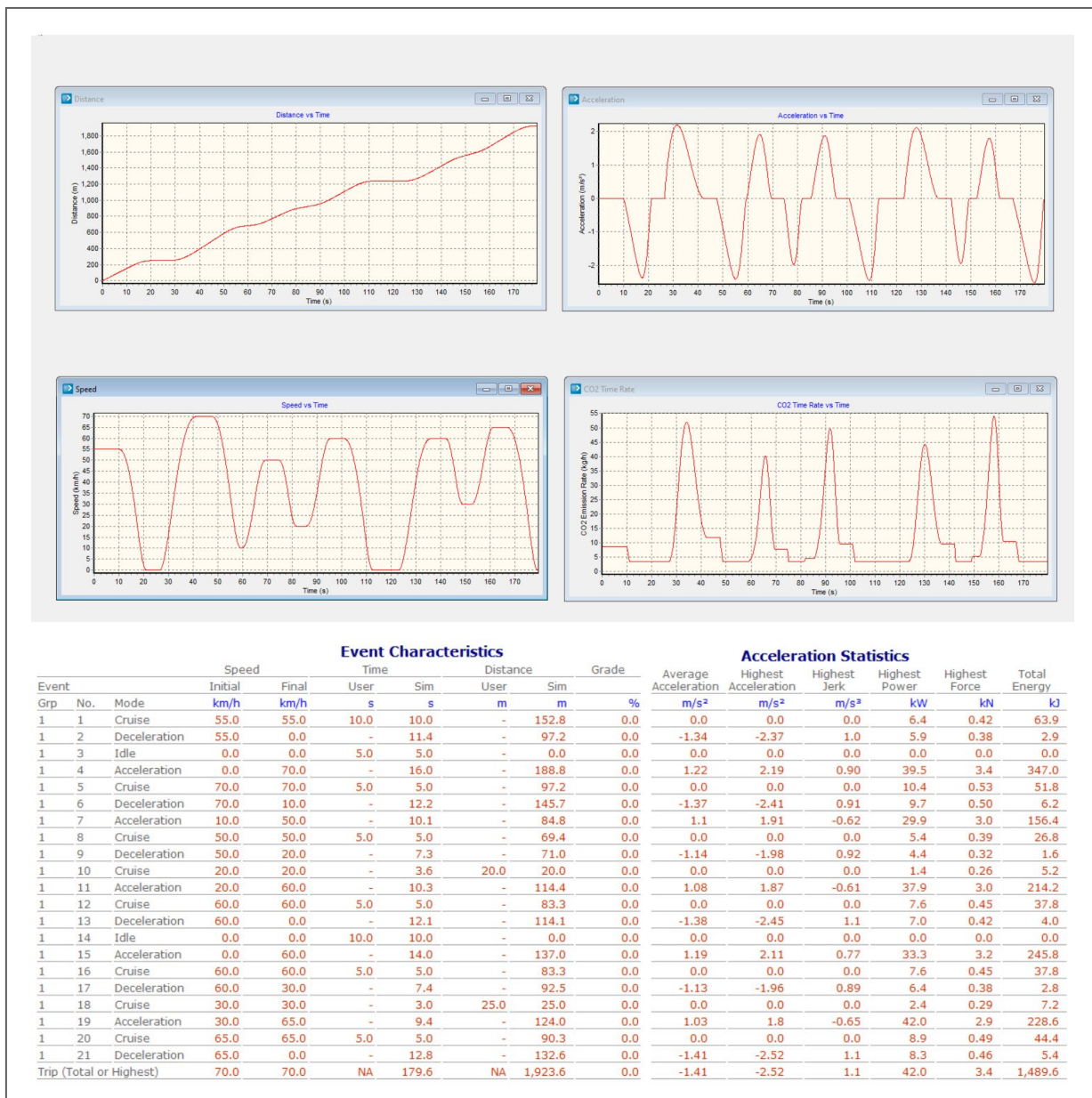
Figure 5 - Drive Cycles for detailed modelling of vehicle paths - an example from SIDRA TRIP
