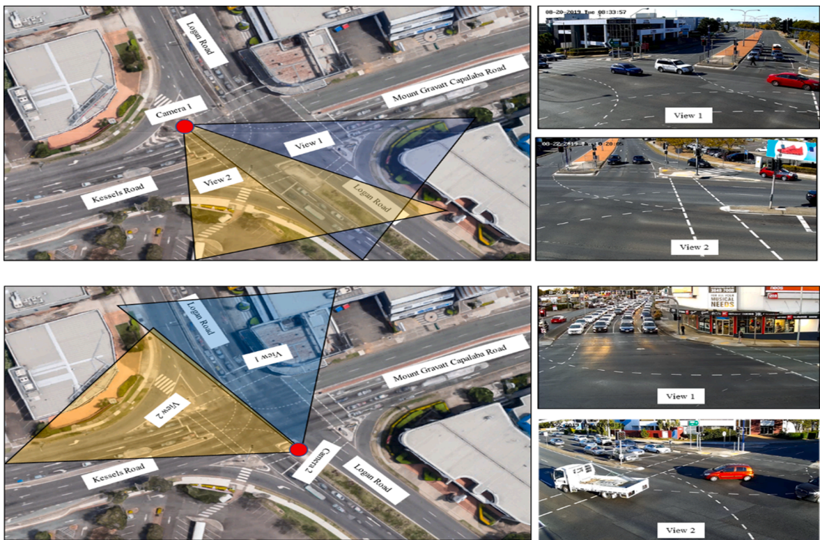
Fig. 4. Camera positions and views from the cameras at the Logan Rd – Kessels Rd Intersection.
